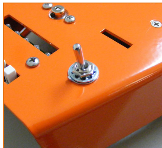
Figure 3.0 – Switch bolted into shell
